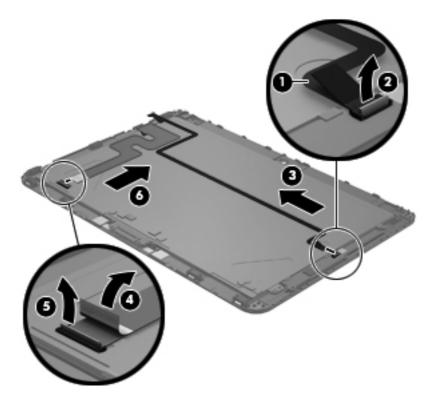
**21.** If it is necessary to replace the home button board and bracket:
